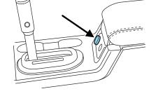
blown, do not use the power point(s) over the vehicle capacity of 12 VDC/180W. If the power point or cigar lighter socket is not working, a fuse may have blown. Refer to *Fuses and relays* in the *Roadside Emergencies* chapter for information on checking and replacing fuses.
